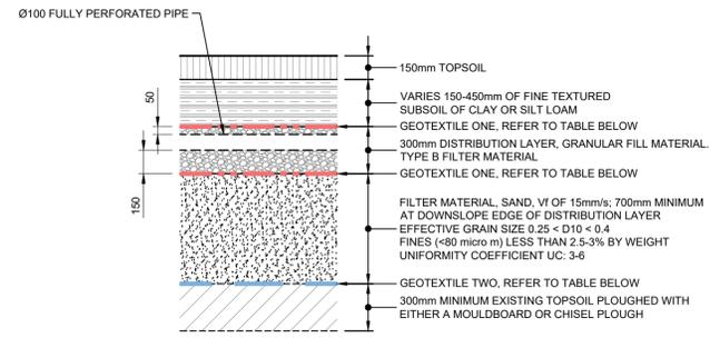
REFER TO NBS SPECIFICATION APPENDIX A FOR DRAINAGE FIELD CONSTRUCTION METHOD
