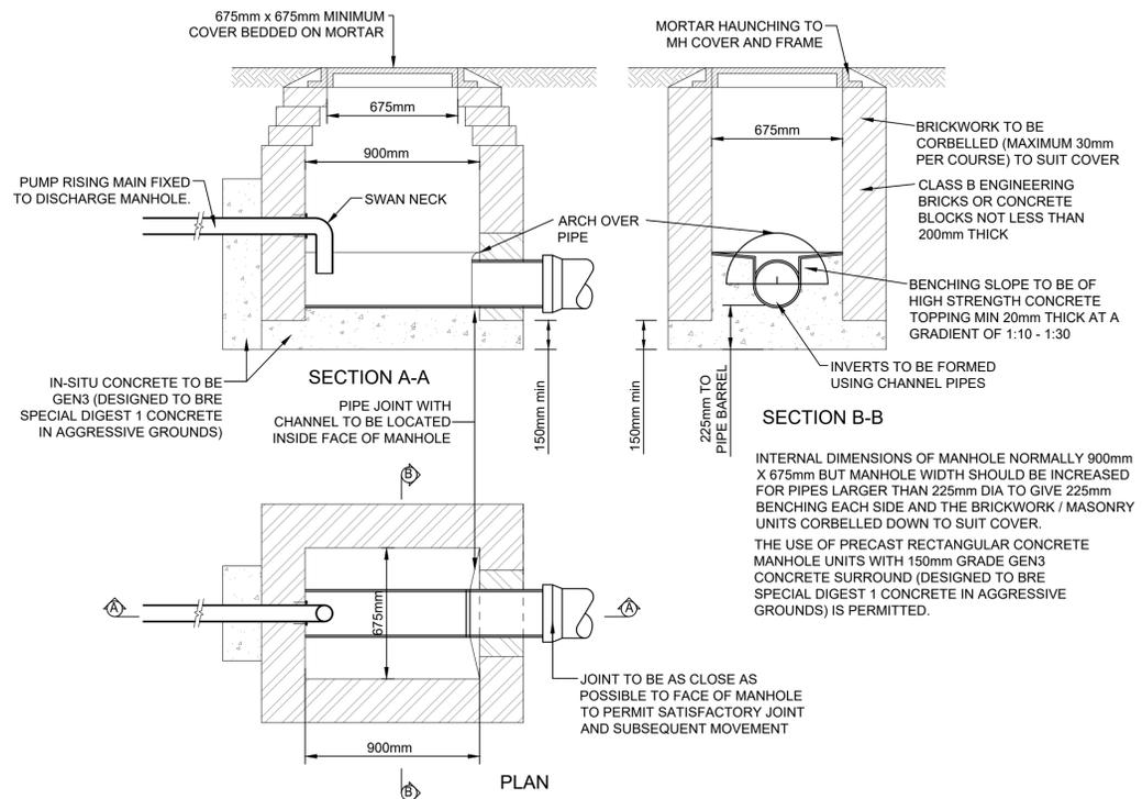
**PUMPED RISING MAIN DISCHARGE MANHOLE DETAIL - TYPE D**
